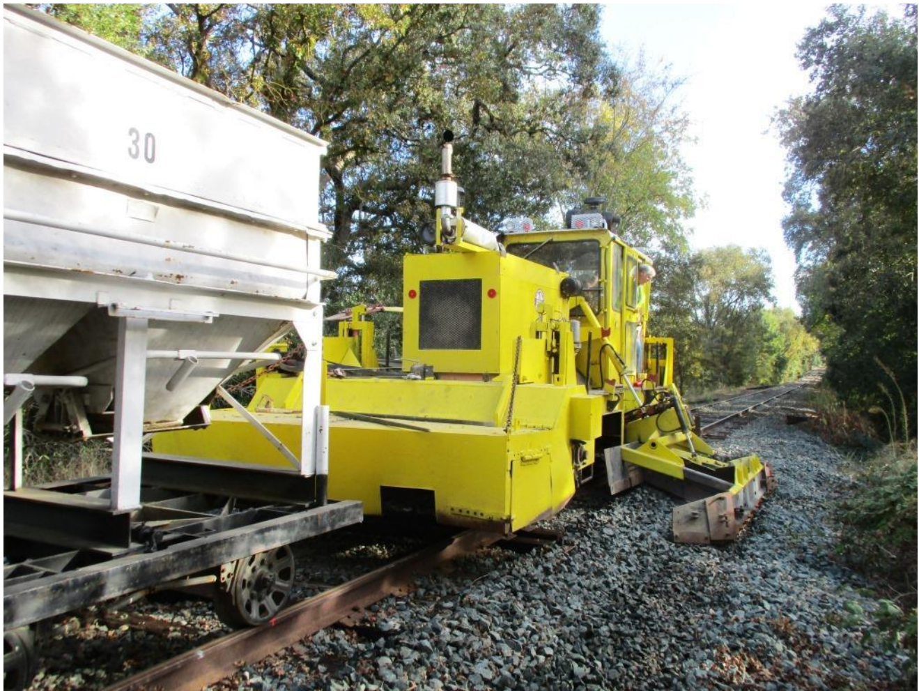
As the regulator passes, it leaves a nice, smooth layer of rock in its wake
